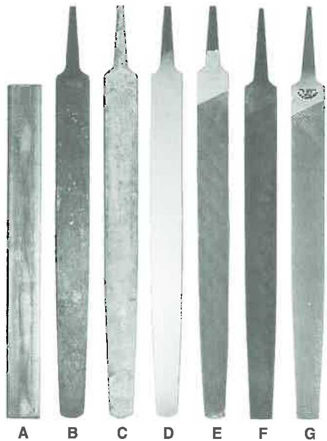
Figure 6-54. Steps in manufacturing a file. A—Steel bar cut to correct length. B—Bar forged to shape. C—Blank after it has been annealed. D—Annealed blank straightened and ground smooth. E—Teeth cut on blank. F—Blank trimmed and coated for heat treatment. G—Completed file cleaned and inspected. (Nicholson File Co.)
