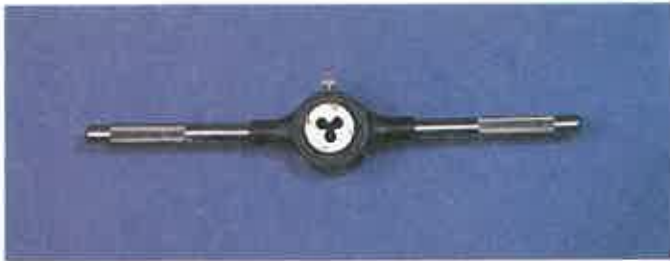
Figure 6-89. The die is held in a die stock.
