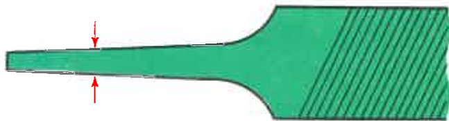
Figure 6-56. File handle hole should be equal in diameter to width of file tang at the point indicated.
