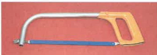
Figure 6-43. A typical hacksaw.
