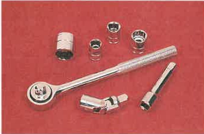
Figure 6-27. A typical socket wrench and sockets. The wrench has a right- and left-hand ratchet mechanism.
