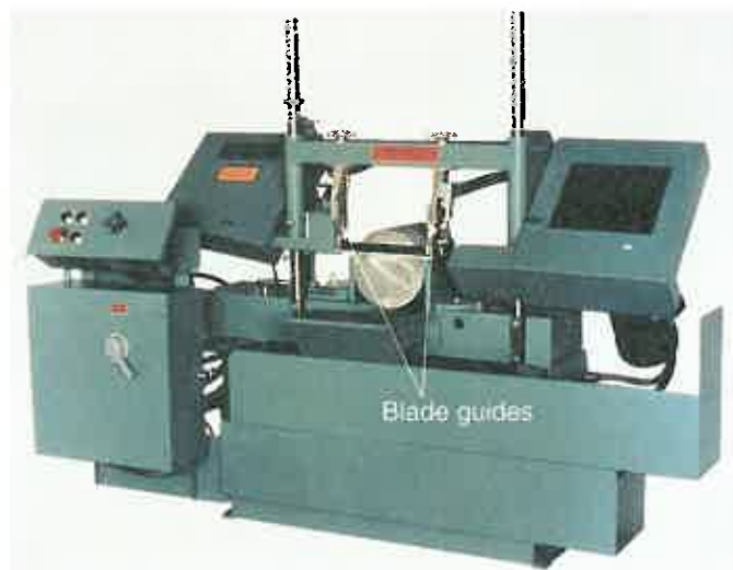
Figure 12-14. Adjust blade guides to provide adequate blade support; otherwise, blade will not cut true. (W.F. Wells)
