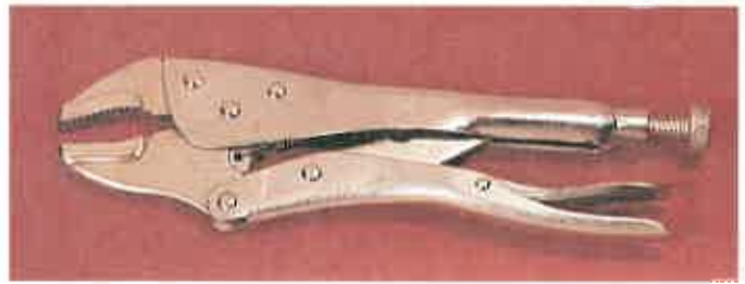
Figure 6-14. Adjustable clamping pliers can be locked on work of different sizes.
