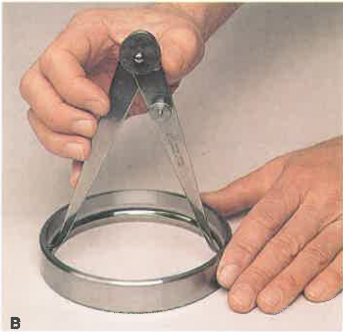
Figure 4-56. Using outside and inside calipers. (L. S. Starrett Co.)
