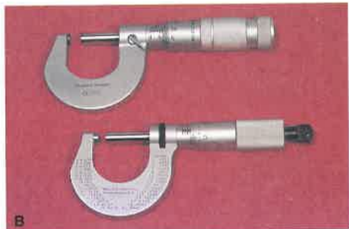
Figure 4-6. The micrometer caliper, past and present. A—A drawing of the Système Palmer measuring device. B—These modern micrometer calipers operate on the same principle as the original 1848 invention.
