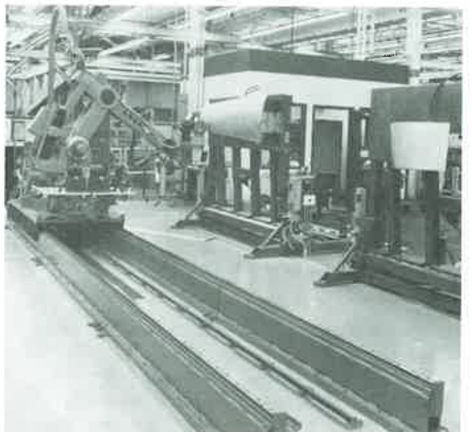
Figure 10-12. This robotic drilling machine moves between workstations on rails. (Northrop-Grumman Corp.)
