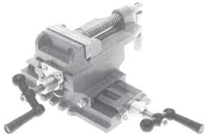
Figure 10-41. A cross-slide vise permits rapid alignment of work for drilling.
