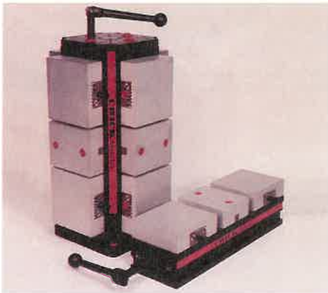
Figure 8-13. Special fixture holding devices for machining centers and other CNC machine tools. Workholding pockets are cut directly into the jaw blocks. Pivoting the vertical setup will bring the next set of workpieces into position. (Chick Machine Tool, Inc.)
