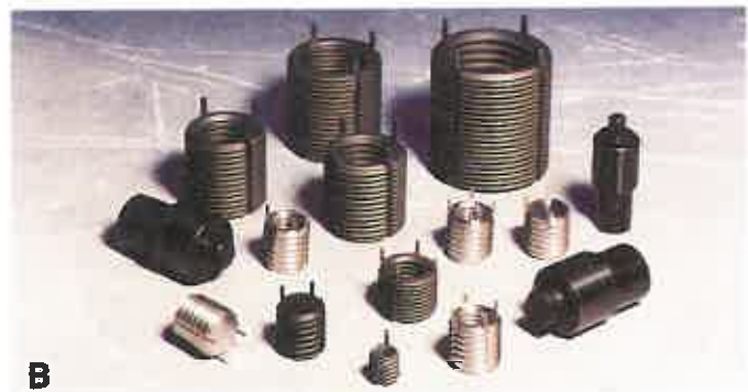
Figure 7-24. Thread repair inserts. A—An insert is frequently used to replace damaged or stripped threads in a part. (Heli-Coil Corp.) B—These keylocking inserts can be easily installed or removed without special tools. They are available in both carbon steel and stainless steel. (Jergens, Inc.)
