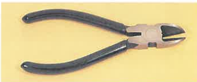
Figure 6-9. Diagonal pliers will cut flush with a surface.
