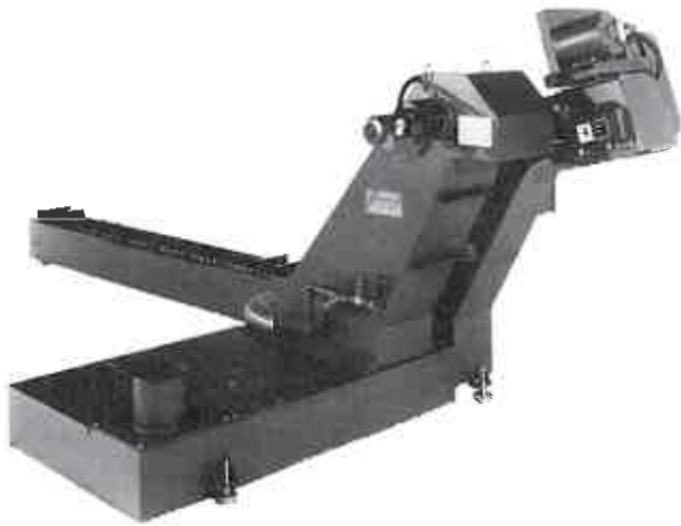
Figure 9-4. This powered conveyor system moves chips away from a machine's cutting area. A rotating drum filter is used to separate chips and metal particles as fine as 50 microns from the cutting fluid. The filtered fluid is recycled to the machine at rates of up to 30 gallons per minute. (Jorgensen Conveyors, Inc.)
