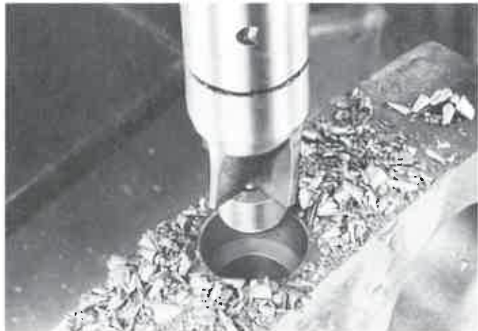
Figure 10-15. Counterboring is done to prepare a hole to receive a flange- or socket-head screw. (Clausing Industrial, Inc.)
