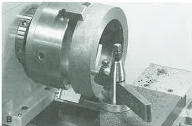
Figure 13-50. Work-holding methods. A—Work being machined between centers. B—Work held in a chuck for machining. (Clausing Industrial, Inc.) C—Work being machined while held in a collet. D—Work bolted to a faceplate for machining.
