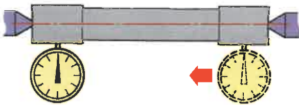
Figure 13-64. Using a test bar and dial indicator to check center alignment.
