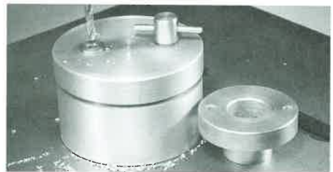
Figure 8-5. With this circular type drill jig, a pin is placed in first hole after it is drilled. This holds the workpiece in position when drilling the second hole. Note the base plate that provides clearance for the drill as it breaks through the workpiece.
