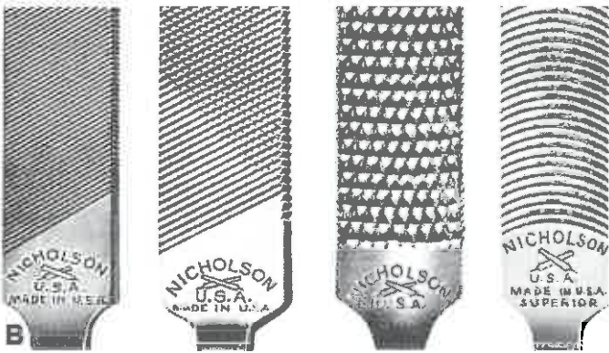
Figure 6-55. File classifications. A—Blunt and tapered files. B—Single-cut, double-cut, rasp, and curved-tooth files.
