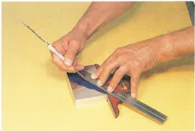
Figure 5-23. Angular settings on layouts can be made with the protractor head and rule of the combination set.
