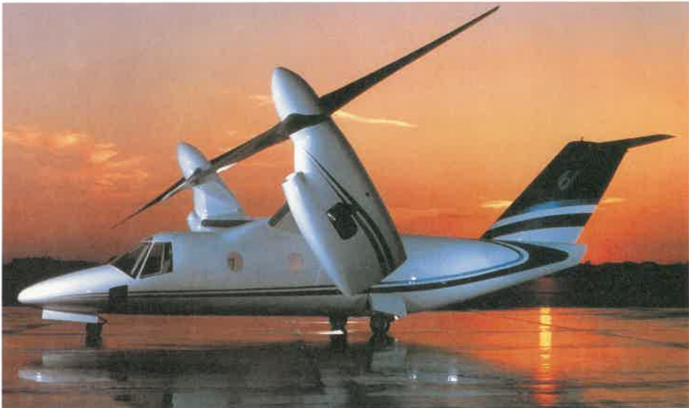
The Bell 609 is the latest design for transporting people in and out of inner city locations. After a helicopter-like take-off, the blades transition into a horizontal position and the 609 flies like a conventional aircraft. The blades are returned to an upright position for a vertical landing. In addition to the use of conventional-type fasteners, high-strength adhesives are used extensively in its manufacture. (Bell Helicopter/ A Subsidiary of TEXTRON, Inc.)
