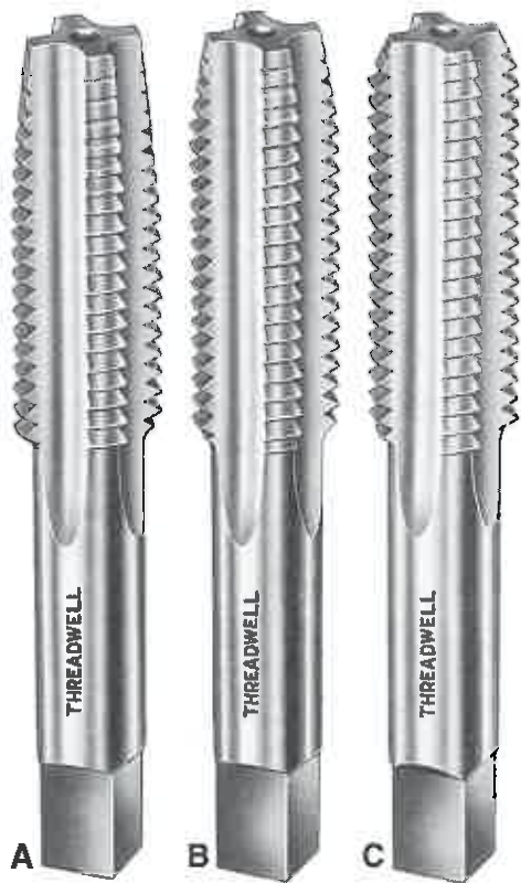
Figure 6-78. Standard hand taps. A—Taper for starting thread. B—Plug tap for continuing thread after taper tap has cut as far into hole as it can. C—Bottoming for continuing threads to bottom of a blind hole. (Threadwell Manufacturing Co.)
