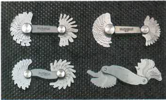
Figure 4-51. Screw pitch gages are made for both inch-based and metric threads. (L. S. Starrett Co.)
