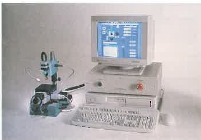
Figure 10-89. CNC microdrilling machine with a point-to-point programmable control system. The table has 2" × 2" (50 mm × 50 mm) travel with an accuracy of 0.0001" (0.0025 mm). Variable speed control for the drill head motor is controlled directly from the computer. (Minitool Inc.)
