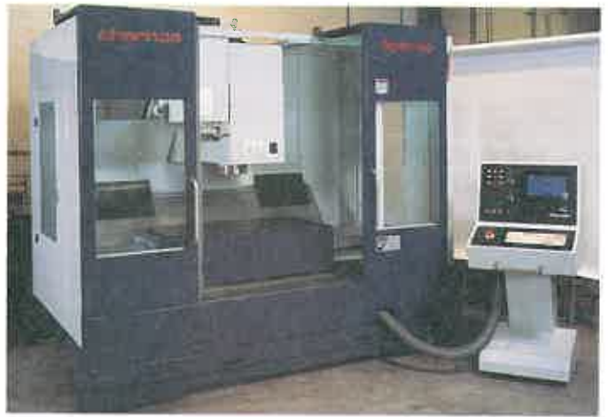
Figure 10-11. Vertical machining center can be programmed to drill holes as part of a machining sequence. No drill jigs are required. Computer numerical control (CNC) is used to set drill position and speed. (Shamo Corp.)
