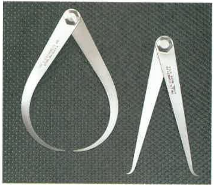
Figure 4-54. Inside and outside calipers. (L. S. Starrett Co.)
