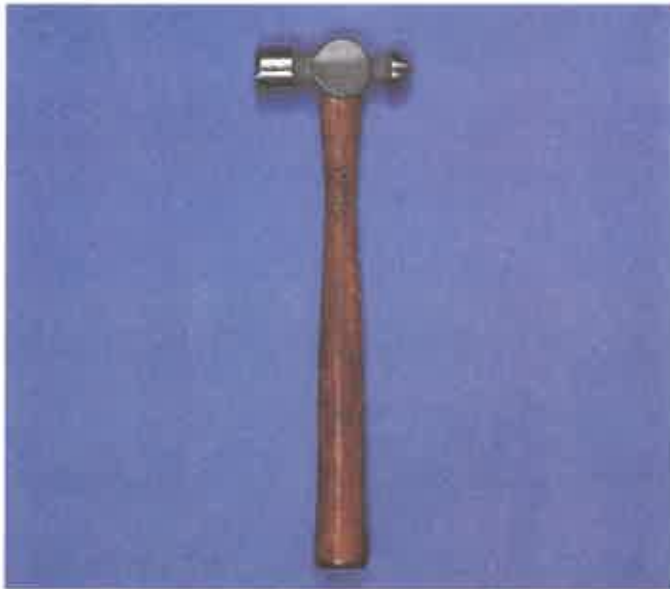
Figure 6-35. The ball-peen hammer is most common type in a machine shop.
