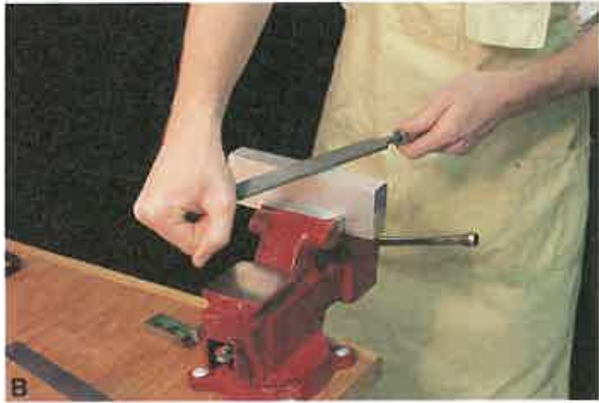
Figure 6-66. Holding a file. A —The proper way to hold a file for straight or cross filing. B —Holding method used to apply the additional pressure required when a considerable quantity of metal must be removed.
