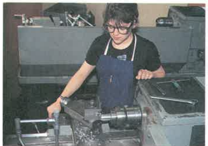
Figure 2-3. This trainee is properly dressed for the job she is doing. She is wearing approved eye protection and a snug-fitting apron. The machine was carefully checked before she began to operate it. (Millersville University)
