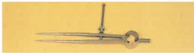
Figure 5-3. A divider is used to mark lines, arcs, and circles.
