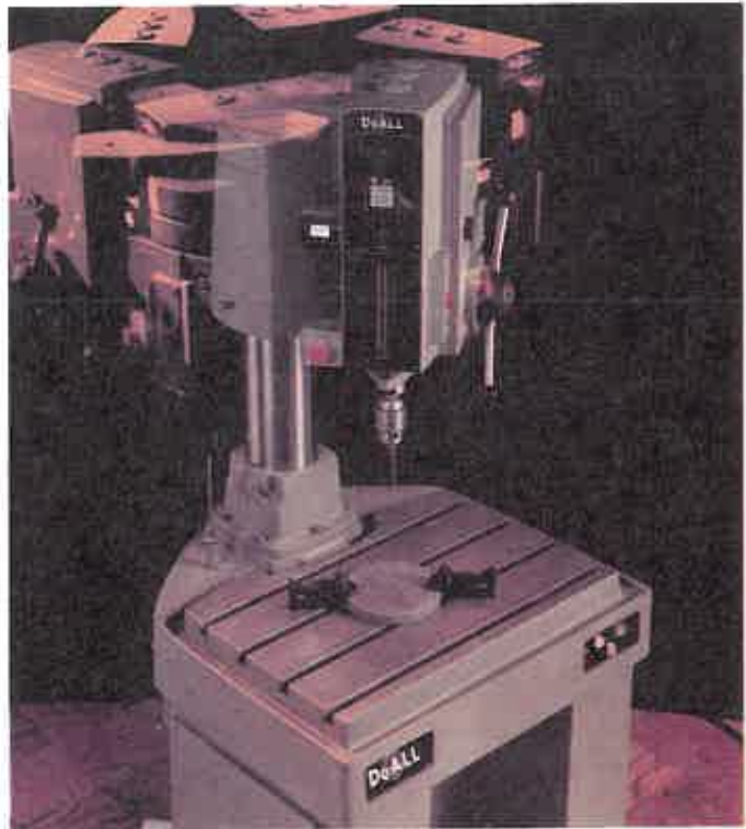
Figure 10-7. Bench radial drill press. (DoALL Co.)
