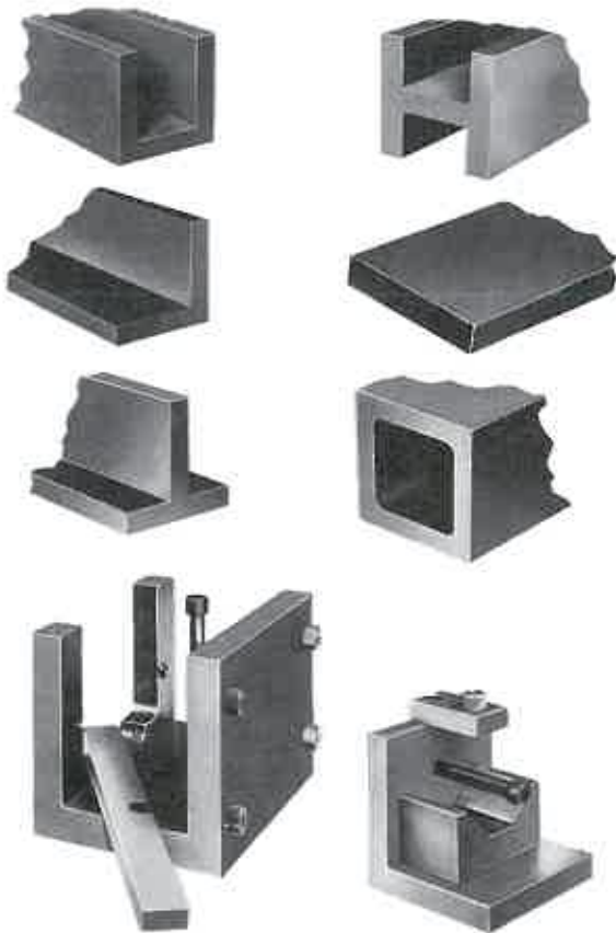
Figure 8-12. Standard cast iron shapes are machined parallel and square to save time and money in both designing and building jigs and fixtures. Sections of different shapes can be bolted together to form complex holding devices. Two completed units are shown at bottom of illustration. (Ex-Cell-O Corp.)
