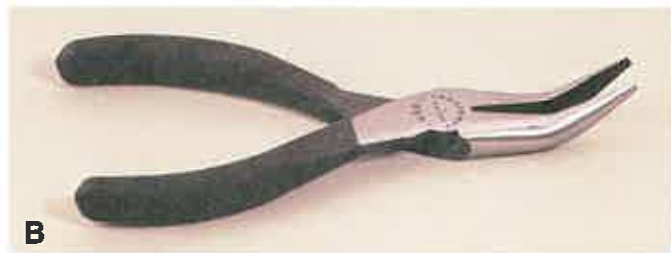
Figure 6-12. Needle-nosed pliers. A —Straight pliers can be used to grasp smaller hard-to-reach objects. B —Curved pliers are helpful when working in areas with limited space.
