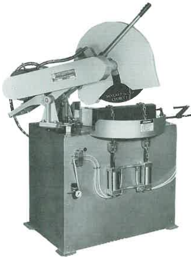
Figure 12-17. An industrial abrasive cutoff saw. (Everett Industries, Inc.)
