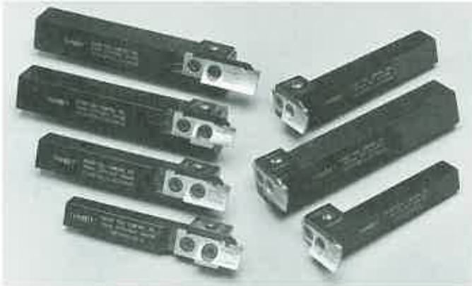
Figure 13-96. Typical straight and offset tool holders for parting and grooving. They use replaceable carbide inserts, which are more wear resistant than conventional high speed tools. (Kaiser Tool Co., Inc.)
