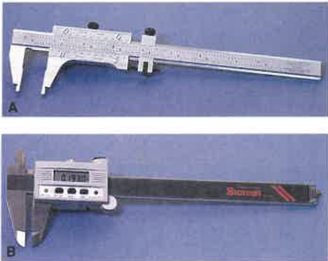
Figure 4-20. Vernier calipers can be used to make very accurate measurements. A—Standard Vernier caliper. B—Modern digital calipers are easier to read than mechanical instruments.
