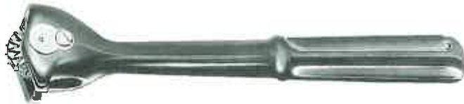
Figure 11-8. A mechanical wheel dresser will true stone face. (Hammond Machinery Inc.)
