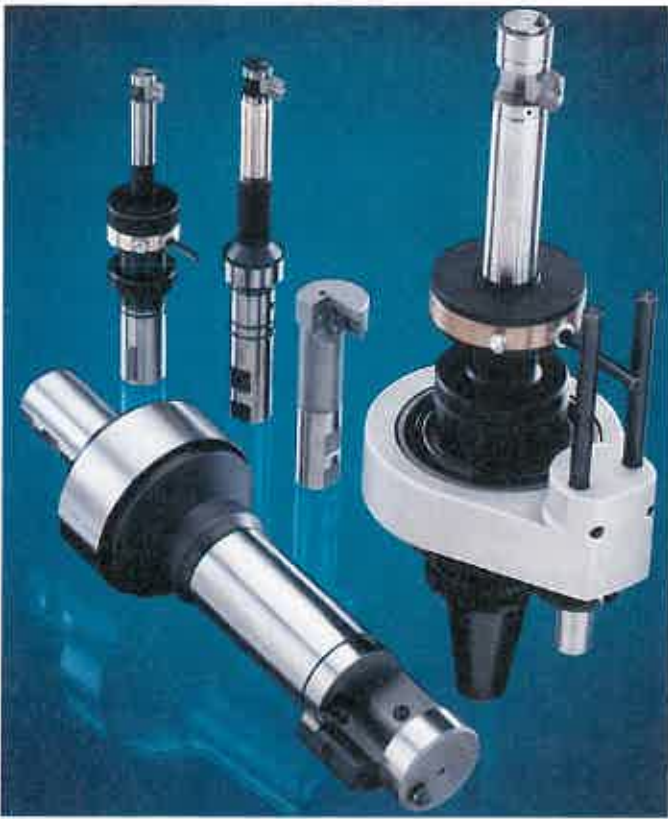
Figure 10-84. Special backspotface and backcounterbore tools are used in situations where conventional tools cannot be inserted. Blade setting can be manual or automatic. Standard tools are available for bores and spotfaces of 0.250 and larger. (Parlec, Inc.)
