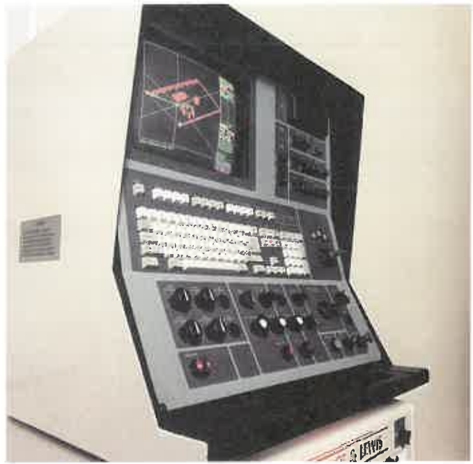
Figure 1-16. CNC machine tools are equipped with on-board computers that permit computer-aided or manual programming. All controls needed for complete machine operation are in one location. A CRT screen displays all important machining information, such as the tool path. (Giddings & Lewis, Inc.)
