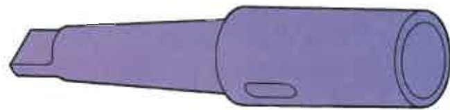
Figure 10-35. A drill socket is used when the spindle is too small for the drill.
