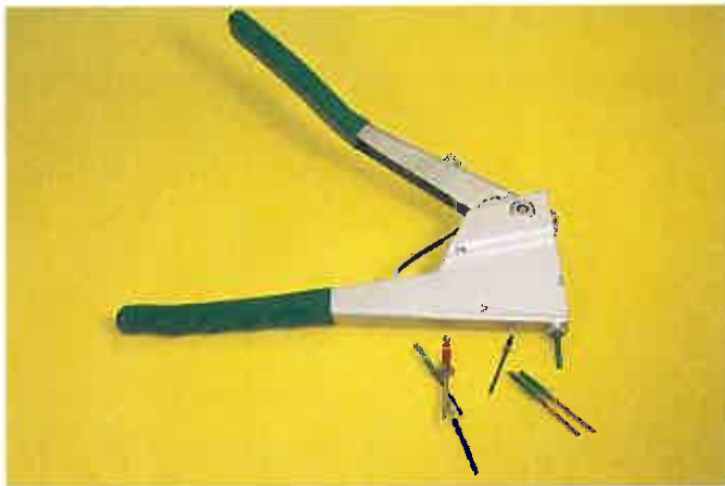
Figure 7-40. A pliers-type rivet gun is used to insert one type of blind rivet.
