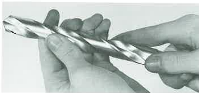
Figure 10-61. One recommended way to hold a drill when it is being sharpened.
