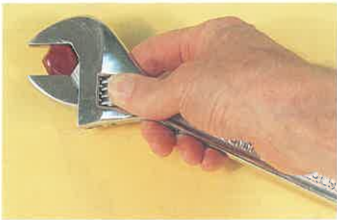
Figure 6-22. A wrench must fit the nut or bolt snugly.
