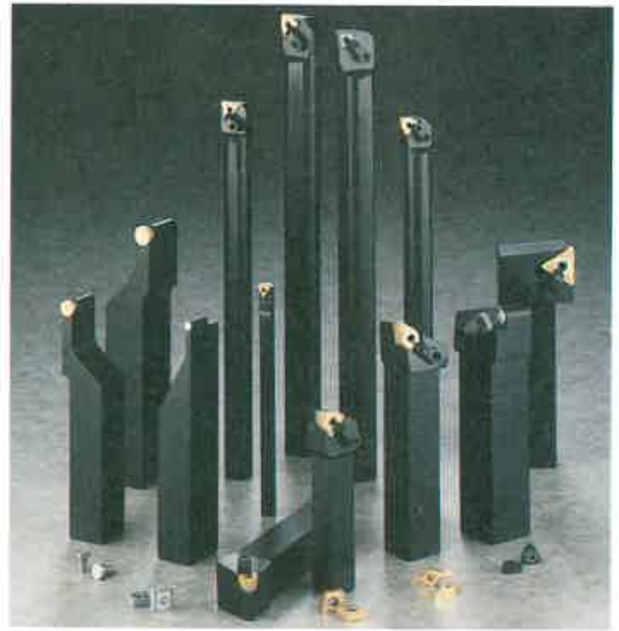
Figure 13-44. A selection of typical holders and replaceable carbide insert cutting tools for the lathe. Each insert has three or four cutting tips. The inserts are clamped in place on the holder, and can be indexed (rotated into position) to present a new tip when the one in use becomes dull. (Carbology, Inc.)
