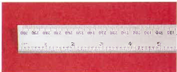
Figure 4-1. This rule can be used to make measurements in both US Conventional and SI Metric units.
