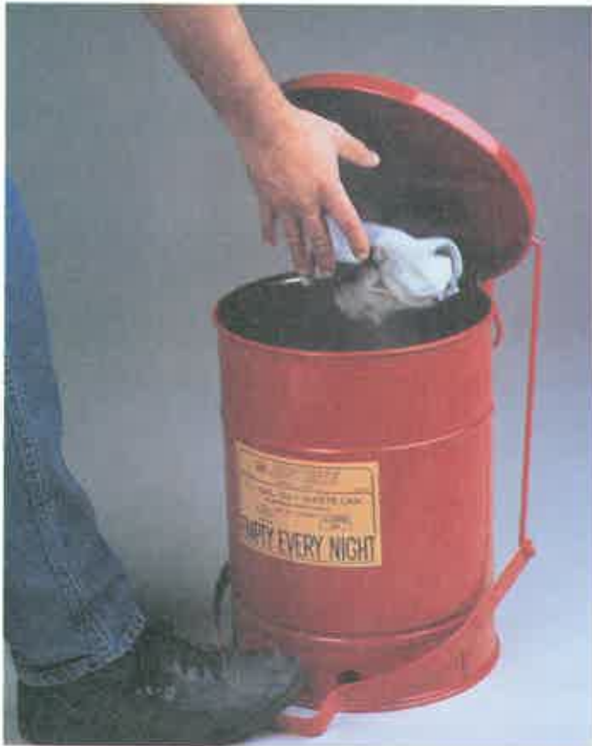
Figure 2-2. Oily rags used for cleaning machines or soaking up spills should be placed in an approved safety container like this one to minimize fire hazards. The container should be emptied daily and contents disposed of properly. (Justrite Manufacturing Company)
