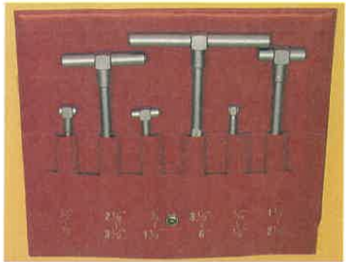
Figure 4-58. A typical set of telescoping gages.
