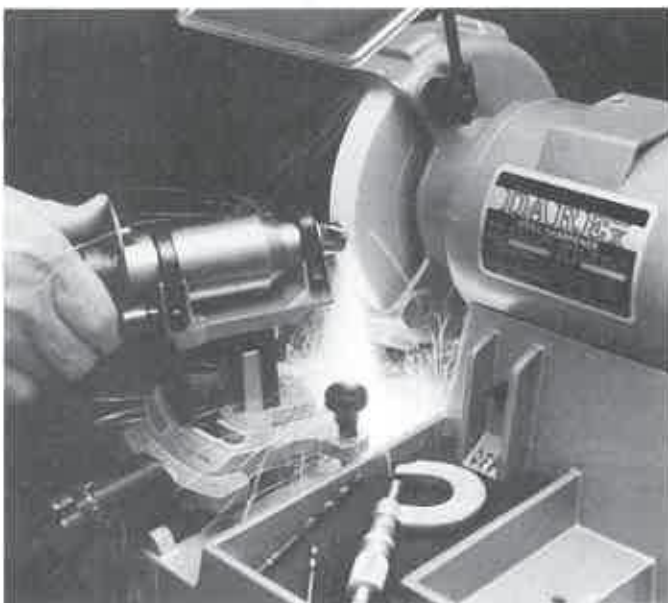
Figure 10-65. A drill sharpening grinder attachment ensures that cutting edges of the drill will be uniform. (Darex Corp.)
