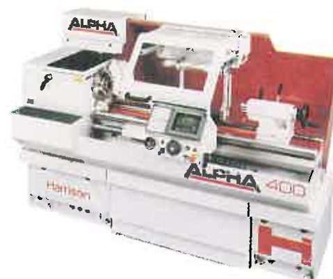
Figure 13-1. Metal-cutting lathes. A—The basic lathe. All controls are operated manually. Most machinists begin their training on this type of lathe. (Jet Equipment & Tools) B—Metal-cutting lathes are some of the most versatile machine tools made. There are many variations of the basic lathe for differing applications. This one is CNC controlled. (Harrison/REM Sales Inc.)
