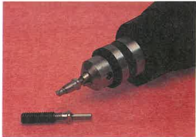
Figure 7-15. The Drill-Out Power Extractor™ combines a drill with an adjustable extractor collar. The drill makes the required-size hole, then the power drill is reversed. This causes the extractor to grip the broken bolt and torque it out. (Alden Corp.)
