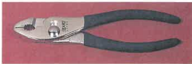
Figure 6-8. Combination or slip-joint pliers are used for holding tasks.
