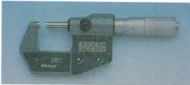
Figure 4-7. This digital outside micrometer can be used to measure in both US Conventional and SI Metric units. (Mitutoyo/MTI Corp.)
