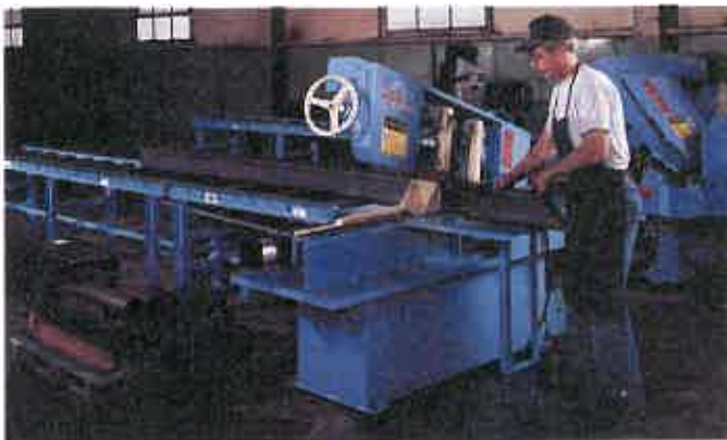
Figure 12-1. The first step in most machining jobs is to cut the stock to the desired length. Measure the cutoff length carefully and observe all safety precautions. (DoALL Co.)
