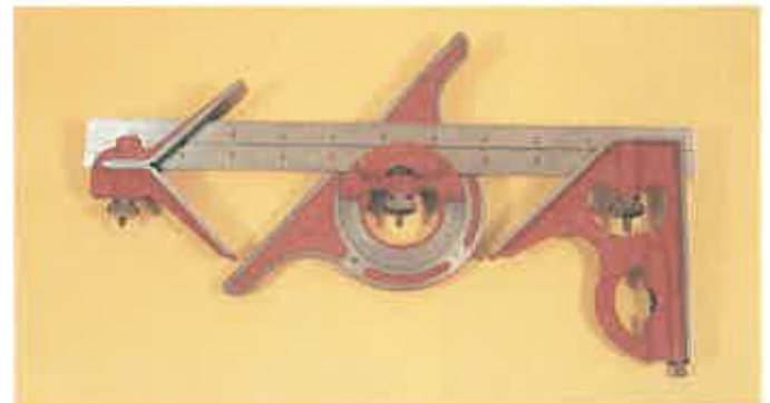
Figure 5-20. A combination set will perform various layout tasks.
