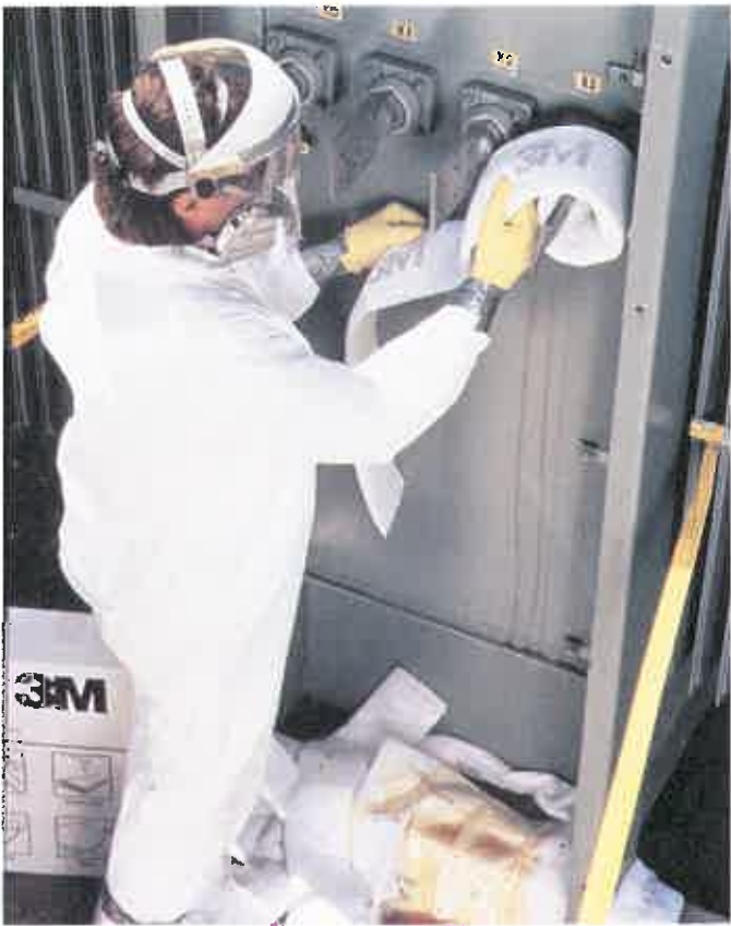
Figure 2-4. This worker in a manufacturing plant is using a special oil-absorbent material to wrap a leaking machine component. Note that the material, which is packaged in roll form, has also been used to soak up oil on the machine base and floor. (3M Company)
