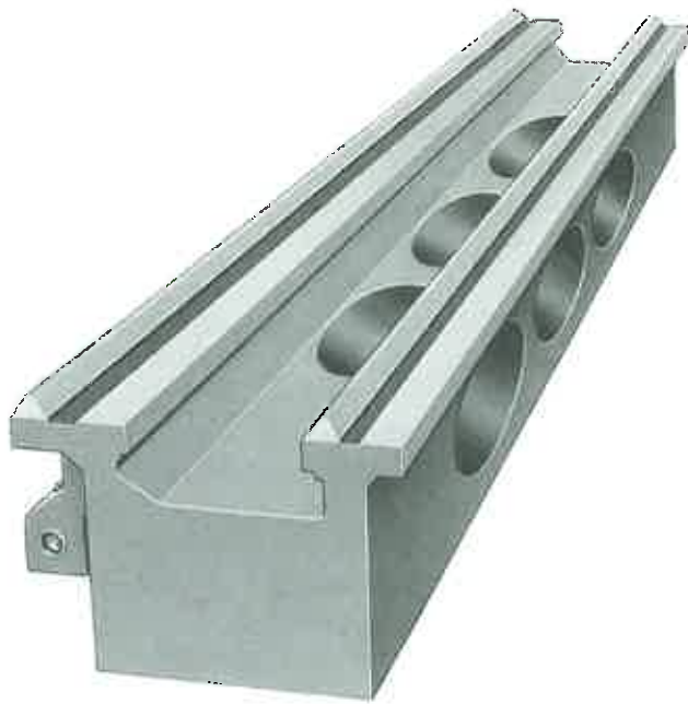
Figure 13-12. The bed is the foundation of the lathe.
