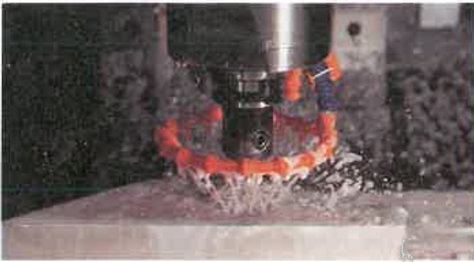
Figure 9-3. Coolant fluid must surround the cutting area for maximum effect. Shown is a modular hose system for applying air and liquids. The units snap together and can be shaped to fit any job. (Lockwood Products, Inc.)
