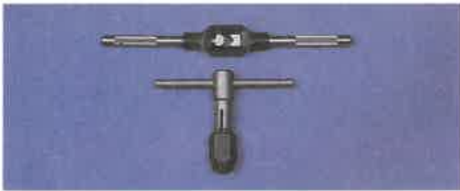
Figure 6-84. Tap wrenches Top—Hand tap wrench. Bottom—T-handle tap wrench.
