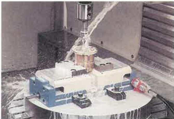
Figure 9-1. For maximum results, coolant should flood the area being machined and cutting tool to provide the most efficient removal of the heat generated. (Kesel/JRM International, Inc.)
