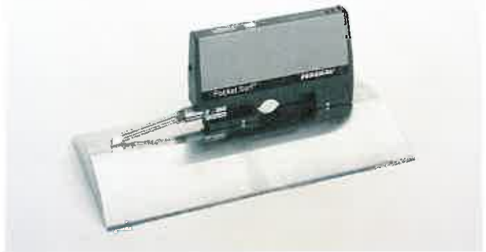
Figure 3-16. Surface roughness is best determined with a profilometer or electronic surface roughness gage. The probe on the unit is moved across the work and measures surface roughness electronically. A digital display presents the measured roughness value in microinches or micrometers. (Federal Products Co.)
