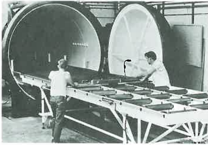
Figure 7-49. This autoclave is used to bond large assemblies, with steam applying heat and pressure simultaneously. The assembly to be bonded is wrapped in a rubber blanket to protect the bond from moisture. (3M Co.)
