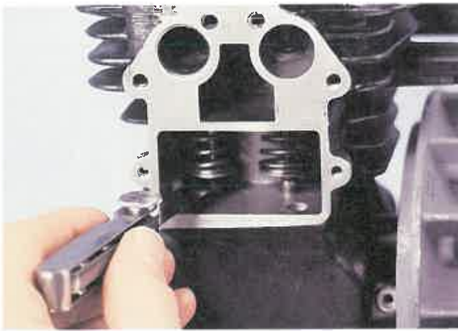
Figure 4-50. A thickness gage is used to check part clearance.
