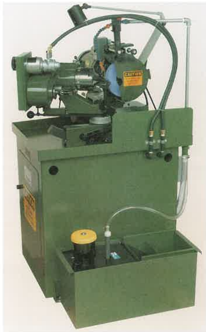
Figure 10-66. A drill and tool grinder with built-in point splitting and web thinning capabilities. The user can choose from a wide variety of drill points. Machines of this type are available in semiautomatic and automatic versions. (Rush Machinery, Inc.)
