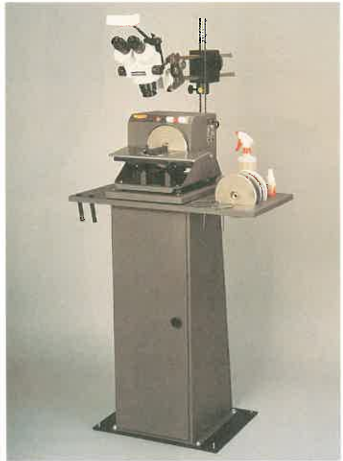
Figure 13-39. A grinder designed for sharpening carbide, cermet, cubic boron nitride, and polycrystalline diamond (PCD) cutting tools. It uses special diamond charged wheels and is fitted with a microscope inspection system.
