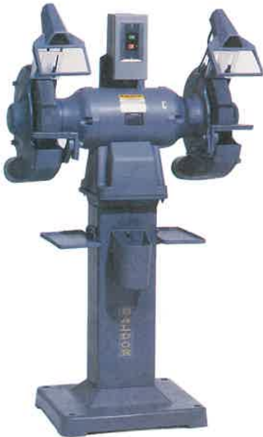
Figure 11-5. This pedestal grinder has a roughing wheel on the left and a finishing wheel on the right. (Baldor)
