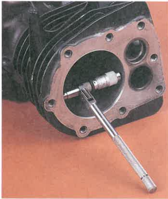
Figure 4-17. Using an inside micrometer. Extension rods can be added to increase the tool's measuring range.
