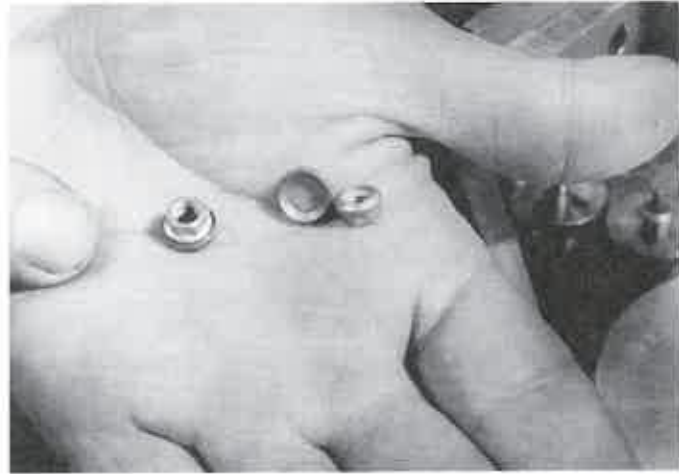
Figure 7-48. Self-aligning nuts used in aircraft are assembled with a cyanoacrylate adhesive. The two part fasteners are assembled automatically and drop onto an indexing table. Setup produces 3600 assemblies an hour. Left—A needle-tip applicator applies a precise amount of adhesive before parts are brought together. Right—Parts after and before assembly. (Loctite Corp.)
