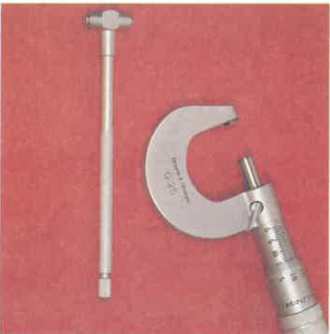
Figure 4-57. A telescoping gage is used with a micrometer.
