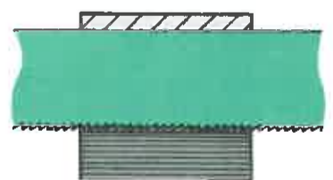
Fine pitch, no chip clearance, teeth clogged
