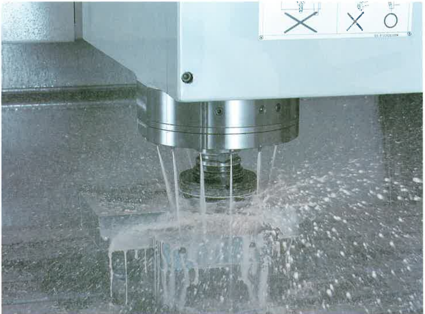
Some machine tools are designed with built-in fluid delivery systems that surround the cutting area, flooding it with coolant to remove heat and flush away chips. In other machines, the delivery system consists of separate nozzles and tubing. (Sharno Corp.)
