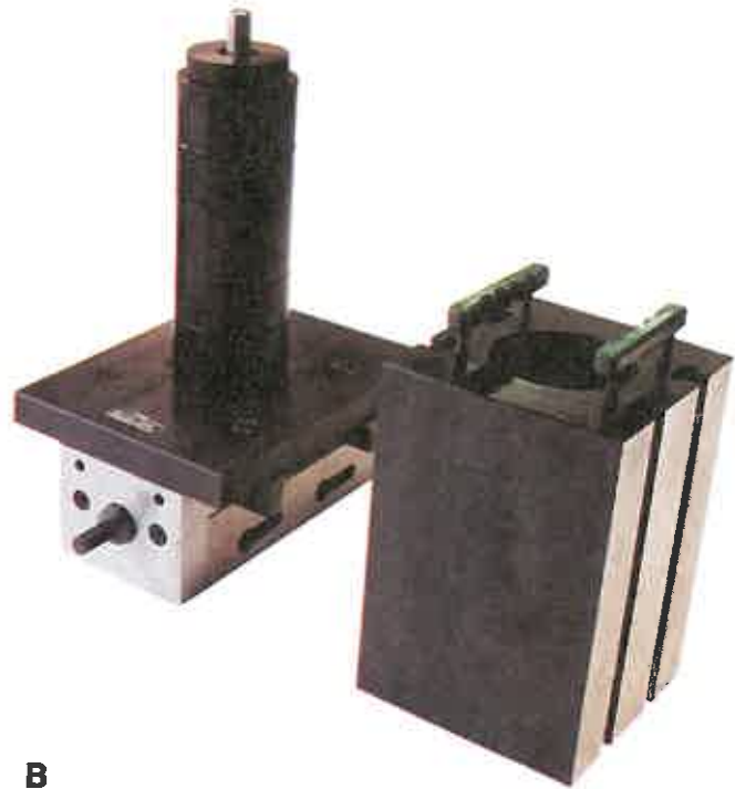
Figure 8-14. "Tombstones" are a common fixture-holding device used with machining centers and other CNC machine tools. They are made from heavy castings and are precisely machined. A—A typical tombstone intended for mounting on a machine's worktable. Fixtures are mounted directly onto the tombstones. The tombstone may be blank, as shown, have drilled and tapped mounting holes, or use T-slots for mounting fixtures. B—A modular tombstone system consisting of a receiver module and mating tombstone modules. An expansion mechanism on the receiver's centerpost allows the tombstone module to be rotated, then locked in position. The assembly at the bottom of the receiver module is a dovetail adapter that allows the assembly to be locked in a standard machine vise. The receiver module can also be bolted directly to the worktable. (Interfen Products Corporation)
