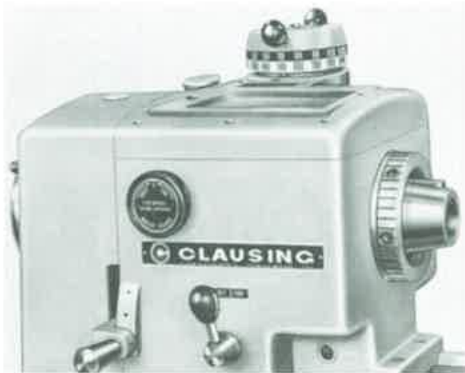
Figure 13-8. The headstock is the driving end of lathe. (Clausing Industrial, Inc.)
