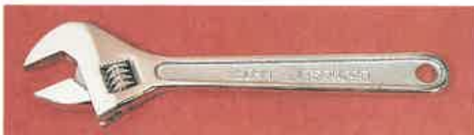
Figure 6-20. An adjustable wrench is handy when a full wrench set is not available.
