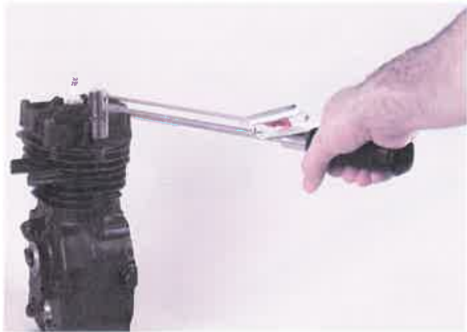
Figure 6-17. Torque-limiting wrenches are used when fasteners must be tightened to within certain limits to prevent undue stresses and strains from developing in the part.
