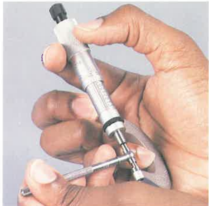
Figure 4-60. After removing the locked telescoping gage, measure it with a micrometer.
