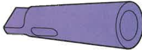
Figure 10-34. A drill sleeve is needed when the drill is too small for the spindle.
