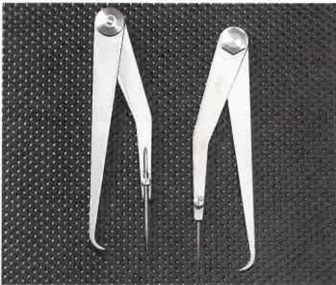
Figure 5-7. A hermaphrodite caliper has a blunt end for the sliding surface and a point for scribing. (L.S. Starrett Co.)
