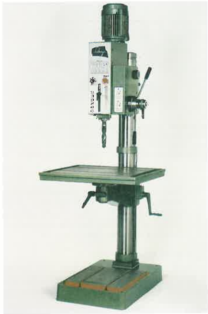
Figure 1-9. A typical 20" variable-speed gear head drill press with power feed. It can drill holes up to 1 1/2" in diameter in cast iron. (Willis Machinery and Tools Corp.)
