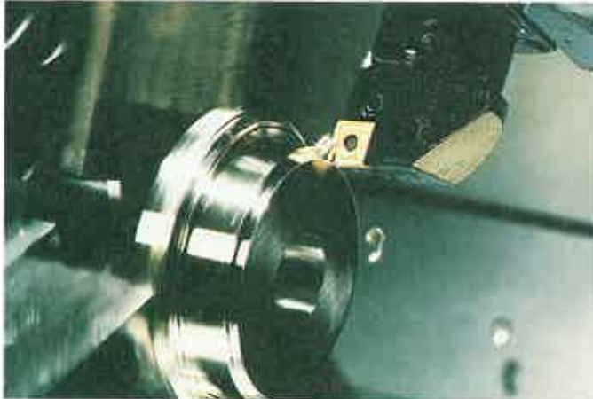
Figure 13-41. Indexable insert cutting tools of carbide or sintered oxides (often referred to as cermets) are mechanically clamped into tool holders to perform cutting tasks. This insert is being used to machine stainless steel. (Sandvik Coromant Co.)
