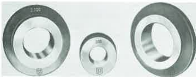
Figure 4-30. Ring gages. The larger sizes are cut away to reduce weight. (Standard Tool Co.)
