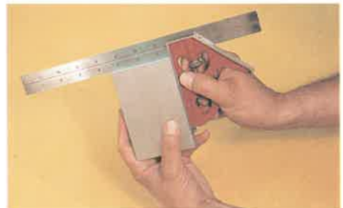
Figure 5-21. The combination set can be used to check squareness and to measure like a depth gage.
