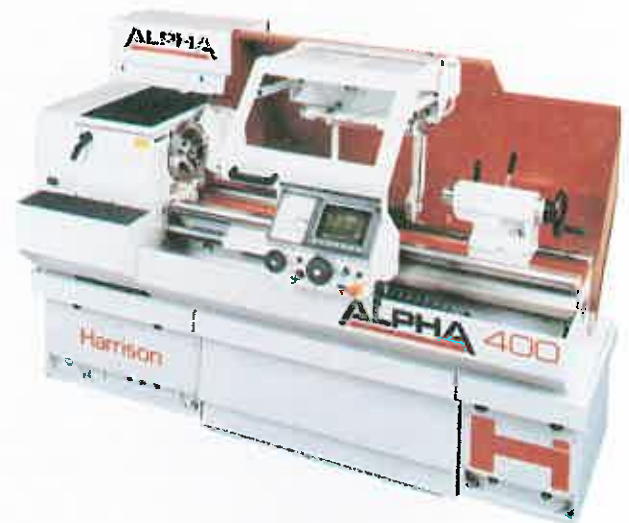
Figure 1-6. A modern lathe using digital technology to perform operations such as maintaining a constant surface speed, automatic threading cycle, automatic radius cutting, and taper turning. Note the safety shield that moves with the carriage. Except those tools that perform nontraditional machining operations, all machine tools have evolved from the lathe. (Harrison/Rem Sales, Inc.)
