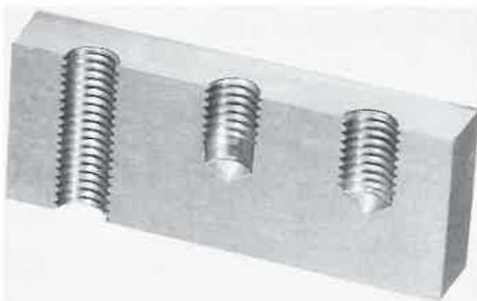
Figure 6-79. Cutaway of metal block illustrates three types of threaded holes. Left—Open or through hole. Center—Blind hole that has been drilled deeper than desired threads. Right—Blind hole with threads tapped to bottom.
