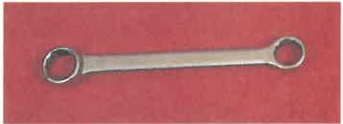
Figure 6-25. A box wrench can handle more torque than an open-end wrench.
