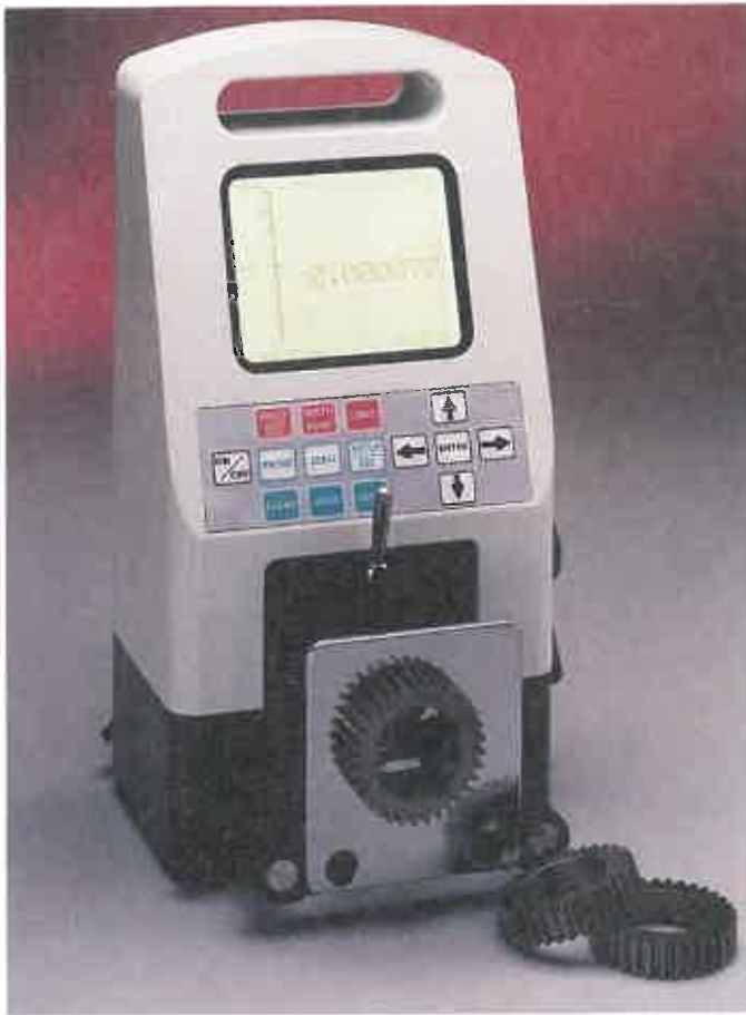
Figure 4-43. This electronic bore gaging system can deliver electronic resolution as fine as 0.00001" (0.0002 mm). Using replaceable gaging probes, the self-contained unit measures diameters ranging from 0.370" to 2.900". It also measures in millimeters. It can be linked to a computer for statistical process control (SPC) data collection. (Sunnen Products Company)
