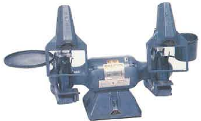
Figure 11-4. A bench grinder can be used for many tasks. Never operate a bench or pedestal grinder unless all safety devices are in place and in sound condition. The tool rest must be properly spaced and eye protection must be worn, even though the grinder has eye shields. (Baldor)
