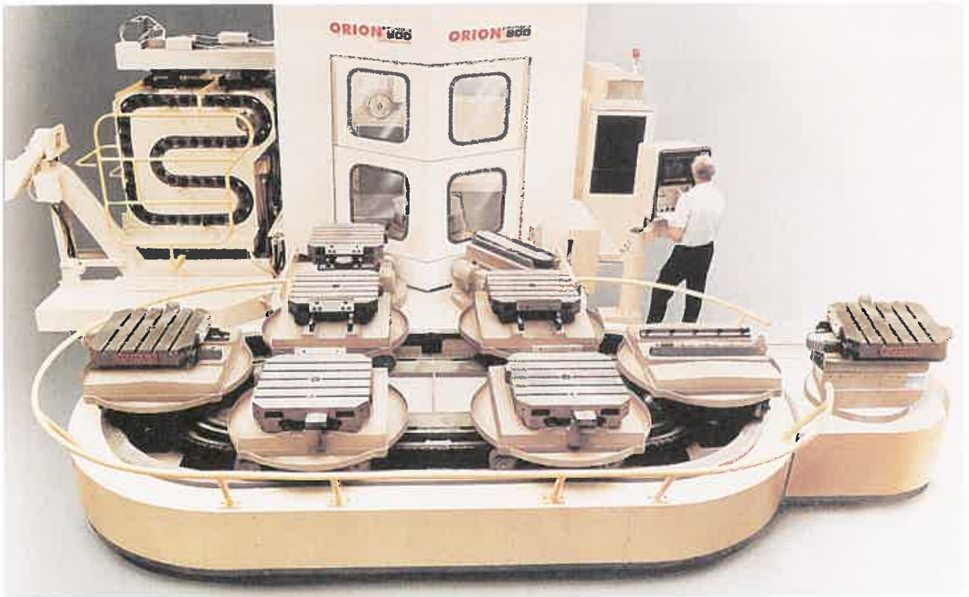
Figure 1-17. A state-of-the-art CNC horizontal machining center (HMC) with multiaxis capabilities. It can handle a wide range of workpiece sizes and materials. The center is fitted with a multiple pallet work storage system (foreground) that automatically transfers workpieces into and out of the machine upon command from the CNC unit. (Giddings & Lewis, Inc.)
