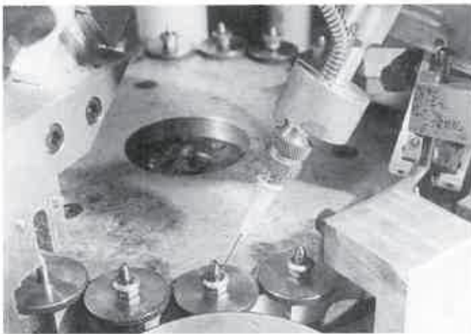
Figure 7-48. Self-aligning nuts used in aircraft are assembled with a cyanoacrylate adhesive. The two part fasteners are assembled automatically and drop onto an indexing table. Setup produces 3600 assemblies an hour. Left—A needle-tip applicator applies a precise amount of adhesive before parts are brought together. Right—Parts after and before assembly. (Loctite Corp.)
