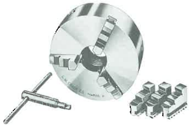
Figure 13-81. The 3-jaw universal chuck automatically centers round or hexagonal stock. (L-W Chuck Co.)
