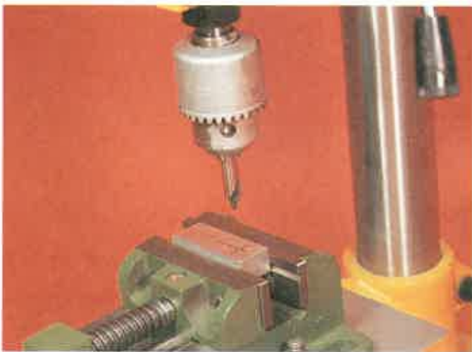
Figure 10-68. After alignment with the wiggler, center drilling will ensure that the drill will make the hole in the proper location.
