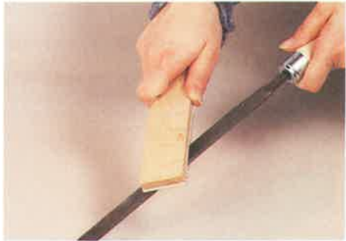
Figure 6-58. Using file card to clean a file.
