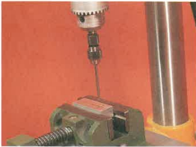
Figure 10-67. It is difficult to align a workpiece with centerlines by eye. To assist in this job, a center finder, or wiggler, is used.
