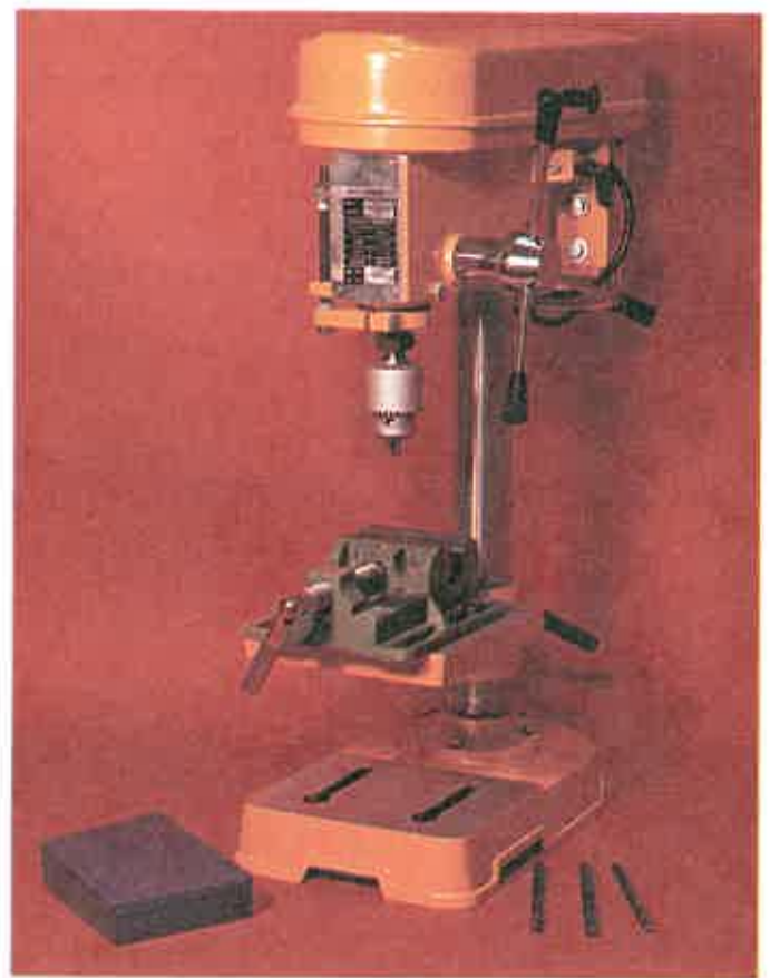
Figure 10-4. A small bench drill press can be very useful.
