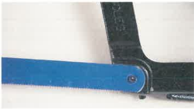
Figure 6-45. A hacksaw blade must be inserted with the teeth pointing away from the handle. This positions it to cut on the forward stroke of the hacksaw.
