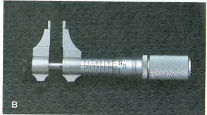
Figure 4-8. Inside micrometers. A—A conventional inside micrometer. B—The caliper jaws on this inside micrometer allow quick and accurate measurements. The divisions on the sleeve are numbered in the reverse order of a conventional outside micrometer. (L. S. Starrett Co.)
