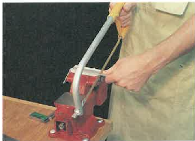
Figure 6-48. Using your thumb to guide the hacksaw blade as the cut is started.
