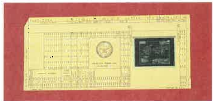
Figure 3-18. The small negative on the microfilm aperture card is enlarged by a photographic process to the desired print size on a microfilm reader/printer. The enlarged print can be verified or confirmed on the view screen.
