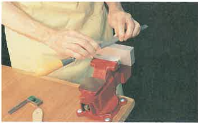
Figure 6-67. Draw filing, when done properly, improves the surface finish.
