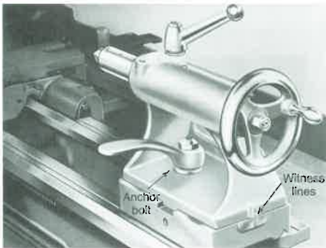
Figure 14-9. The tailstock is usually constructed in two parts. This allows the section mounting the center to be shifted relative to the lathe's centerline. The distance off center, or setover, can be checked by observing the witness lines. (Rockwell International)
