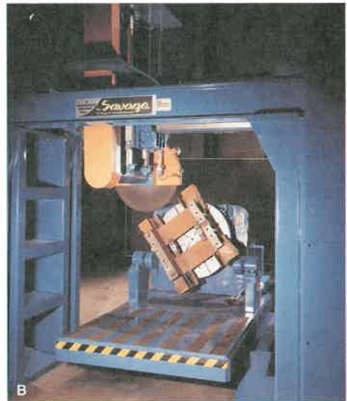
Figure 12-18. Cold circular saws. A—This automated cold circular saw can accept a piece up to 2500 pounds. A laser guide light marks the position of the cut. B—This machine can be fitted with carbide-tipped blades or abrasive disks. (W.J. Savage Co.)
