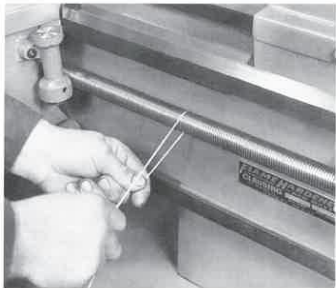
Figure 13-24. This machinist is cleaning lead screw with a piece of cord. The lead screw should rotate at low speed. Do not wrap the cord around your fingers or hands.
