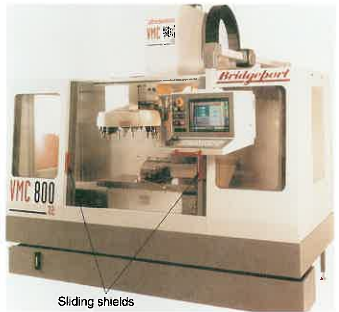
Figure 2-9. Many CNC machine tools use sliding shields over the machining area to protect the machinist from flying chips and vaporized coolant. (Bridgeport Machines, Inc.)
