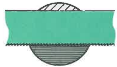
Fine pitch, no chip clearance, teeth clogged
