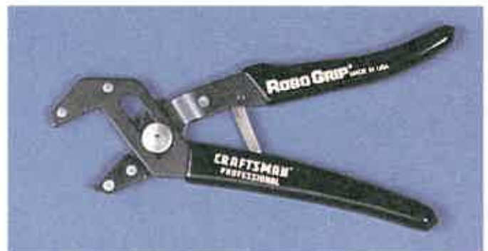
Figure 6-15. The newest type of adjustable pliers offers one-handed operation.
