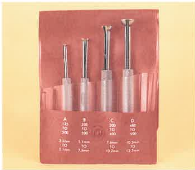
Figure 4-61. Small hole gages are used to measure the diameter of holes that are too small for telescoping gages.
