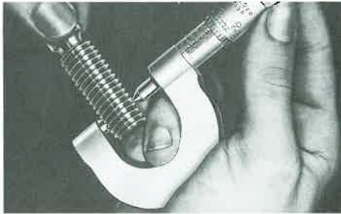
Figure 14-39. A thread micrometer can be used to check cut threads precisely. (L.S. Starrett Co.)
