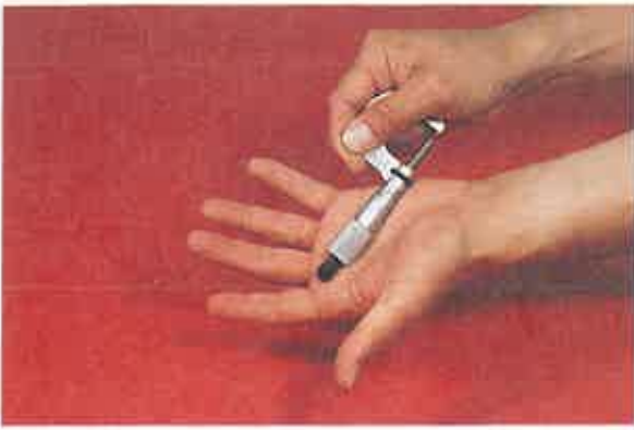
Figure 4-19. Micrometers must be treated carefully. Roll the micrometer thimble on the palm of your hand if the instrument must be opened or closed a considerable distance.
