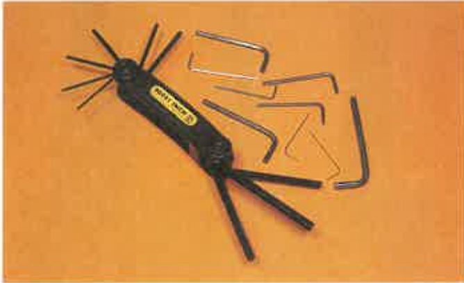
Figure 6-30. Allen wrenches are used with socket-headed fasteners. They are made in both inch and metric sizes.
