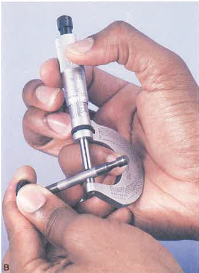
Figure 4-16. Proper technique of handling a micrometer. A—Use very light pressure when turning the thimble. B—When the piece being measured must also be held, position the micrometer as shown, with a finger in the micrometer frame.
