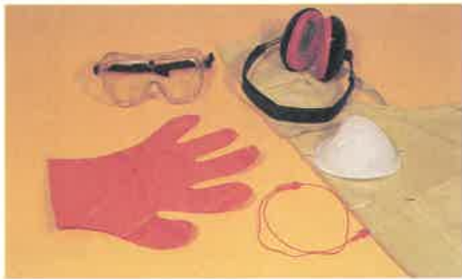
Figure 2-5. Wear appropriate safety equipment. Shown are approved eye protection, an apron to protect clothing, plastic gloves for handling oils and solvents, a hearing protector, earplugs, and a dust mask.
