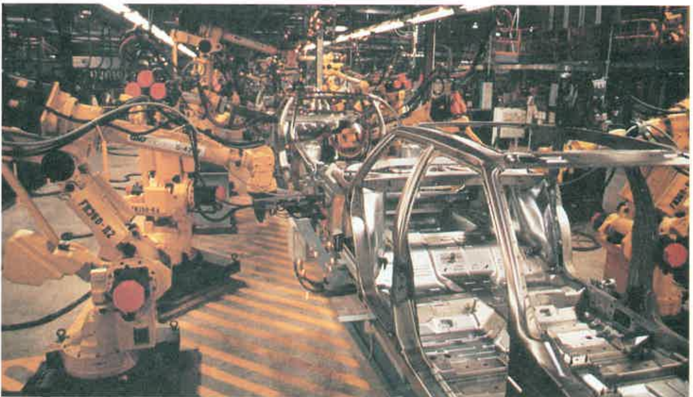
Figure 1-19. The automotive industry makes extensive use of robots for positioning parts, welding, painting, and performing quality control tasks.
