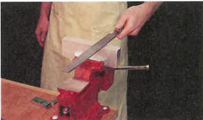
Figure 6-65. Mount work at elbow height for general filing.
