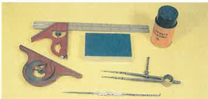
Figure 5-1. A few of the tools needed to make a simple layout.
