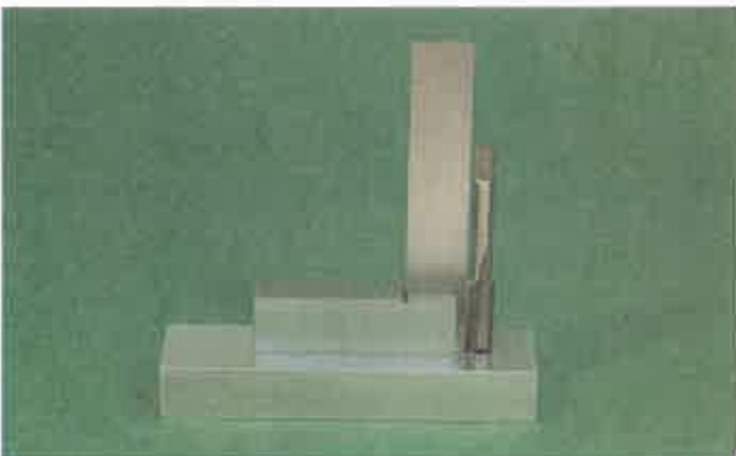
Figure 6-85. A tap must be started squarely with the hole. A quick way to check this is to use a machinist's square.
