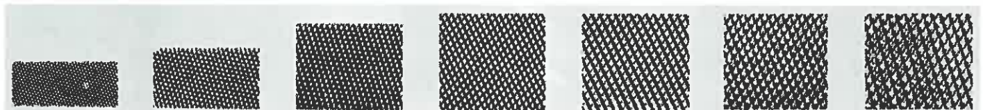
Figure 6-63. Range in coarseness of a typical machinist flat bastard file. File sizes range from 4" (100 mm) to 16" (400 mm). (Nicholson File Co.)
