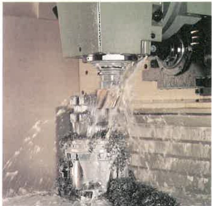
Figure 9-2. An additional function of cutting fluids is to flush away chips from the area where cutting is taking place. (EROWA Technology, Inc.)
