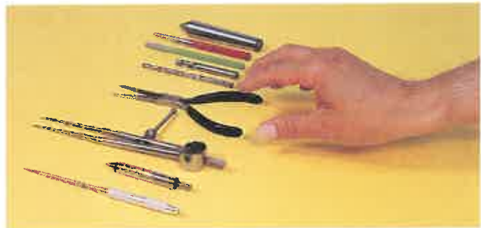
Figure 2-12. Arrange sharp pointed tools on the bench in a way that they will not injure you when you reach to pick them up.
