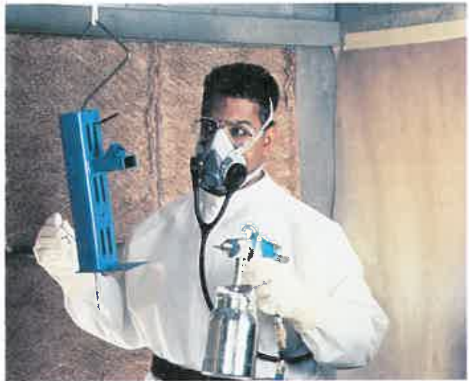
Figure 2-6. Whenever fine airborne mists of oil, coolant, or other materials are present, an approved respirator is required. This spray painter is wearing a respirator supplied with clean air through a tube from a central source. It is also important to use proper eye protection, such as the safety glasses worn by this worker. (3M Company)
