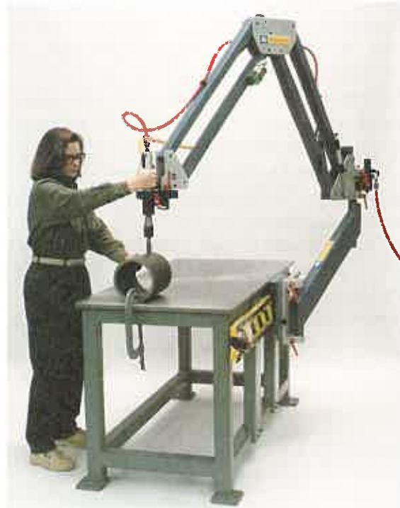
Figure 6-86. Articulated arm power tapper. The machine can be fitted with an auto reverse system (the tap is run out of the hole automatically when the threads are at the proper depth), automatic lubrication of the tap, and a digital depth readout. (Procyon Machine Tools)
